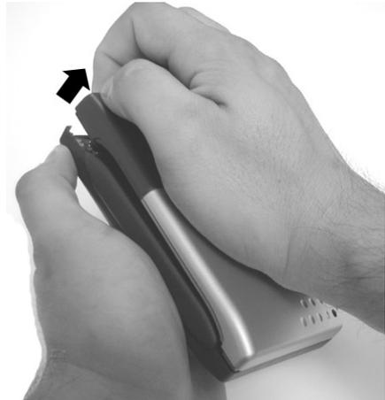
**Note:** The end cap of the enclosure is removable and may come out of its slot. If so, remember to put it back in its slot before replacing the top cover of the enclosure.
