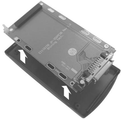
**Step 4:** Look at the hard drive connector pins and observe that there are two groups of such pins. These two groups are separated by a noticeable gap in the sequence of pins. The first group (Group A) has 22 contiguous 2-pin columns (which actually has one pin missing in the middle of one of its rows). The second group (Group B) has just 2 columns of pins and is located at the left end of the drive connector.
